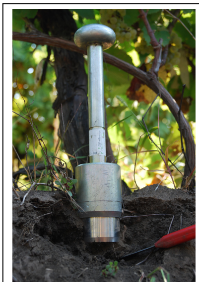
Fig. 2 - Core sampling for bulk density determination
